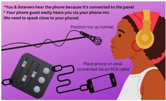
As above, you must connect your phone to either the AUX or PHONE hub via an RCA cable. (Mixer shown just an example of a generic mixer in place of actual MainFM studio mixing panel)
