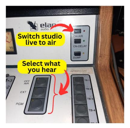
When we go 'ON-AIR' (top right) we are feeding signal to our transmitter which sends our program across the air waves - literally 'on air'. So, to transmit from our studio we need to switch it into the transmission circuit. When we do this the studio is 'ON AIR' – ie we are sending our program to the transmitter. When this button is pushed, the 'ON THE AIR' sign on the wall lights up white.
